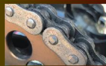
rust on pin/plate surface
