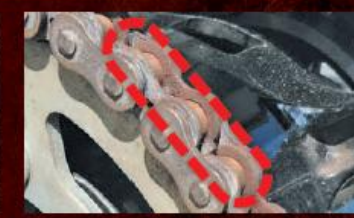
insufficient lubrication, roller wear
