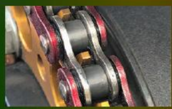
well-lubricated and in good condition
