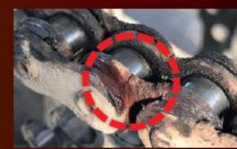
seal ring's deterioration, pin/bushing wear, steel powder oxidizing
