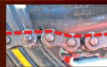
chain not flexure, line misalignment
